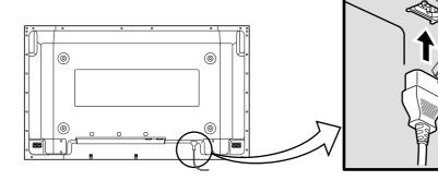
Fix the AC cord plug securely to the Plasma Display with the clamper. (see page 7)
